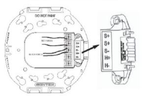
The access holes are provided in the back of the terminal block to allow the voltage to be measured directly without removing the device. Typically this would be done at the end of the line to confirm design criteria. Most measurements will be taken using the S+ and S- locations although access is provided to other locations. Note: Care should be taken to not short the test probes.
