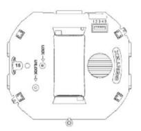
Switch positions 1 and 2 in the down position to select isolated horn and strobe power inputs. Switch 3 selects between temporal or non-temporal tone. Up is temporal. Switch 4 selects between mechanical or high frequency tone. Up is mechanical. Switch 5 selects between high or low dBA. Up is high dBA.
