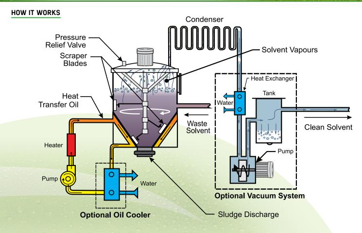
**Vessel Design:** The exclusive 60° cone vessels design allows proper heat distribution and ease of residue removal. This design has more heat transfer area at the top of the cone. As sludge accumulates, it naturally drops to the bottom of the cone leaving the larger surface area at the top to keep on distilling at optimal efficiency. Under these conditions, the sludge is always submerged in solvent and acts as an additional safety feature with reactive materials such as nitrocellulose.
