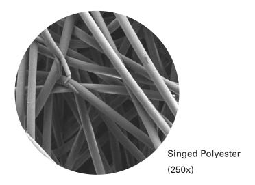
Needled 16 oz. singed polyester felt is a versatile and cost effective filtration media used in pulse jet baghouse dust collectors. The singeing process removes fiber fuzz and creates a more uniform finish, allowing for a better dust cake release than untreated polyester media. This material is strong, abrasion and chemical resistant and good for applications up to 275° F.
