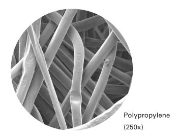
Needled 16 oz. polypropylene felt is a chemical resistant filtration media used in pulse jet baghouse dust collectors. This material exhibits excellent chemical resistivity and holds up in applications with acids, alkalis and/or hydrolysis. It is resistant to bacteria and mildew and is good for applications up to 200° F.
