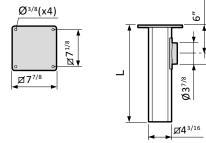
Ceiling bracket, for fitting through beams. The attachment plate is adjustable for the entire length of the aluminum profile. If required, the aluminum profile can be cut during fitting. Ø37/8 Ø<sup>3/8</sup> (x4)
